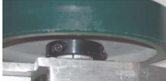
3.) Remove bolt and drive wheel. A wheel puller or other mechanical means may be required to slide the wheel off the motor shaft. Remove old clamp (if any).
