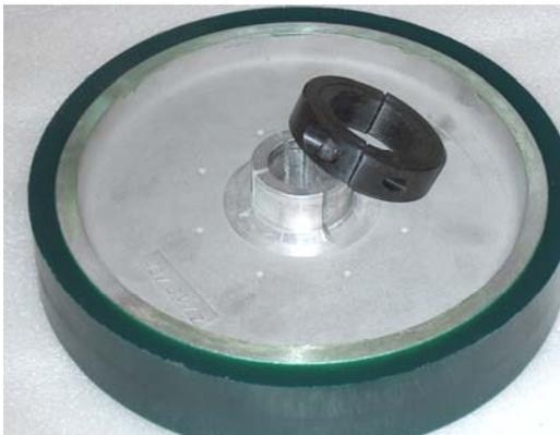
6.) Place the locking collar on the machined inside hub on the replacement wheel (collar splits between hub splits) and lightly tighten. **Be sure the collar is seated against the back of the wheel hub.**
