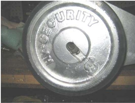
8.) Install new bolt and new washer on wheel/motor assembly.
