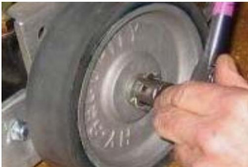
4.) Clean debris from shaft (emery cloth works well), and replace the motor shaft key with the key included in the installation kit.
