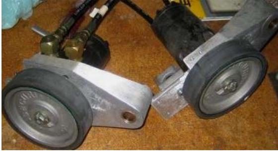
2.) If the old wheel is equipped with a locking collar, loosen the two (2) 3/16" Allen head bolts holding the clamp (requires a wrench at least 4" long for 8" wheels).
